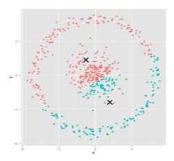
*Note.* K means clusters are most effective when underlying data distributions can be easily grouped into values with similar means, when underlying patterns are non-linear, K means clustering is ineffective. Taken from "K-means clustering is not a free lunch" by David Robinson on Variance explained, January 16, 2015 (retrieved from <u>http://varianceexplained.org/r/kmeans-free-lunch/</u>)
