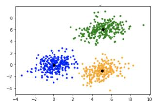
*Note.* K means clusters are most effective when underlying data distributions can be easily grouped into values with similar means. The figure shows an effective clustering method and proper data shape for K means analysis. Taken from "Ideal Clustering" by Savyalholsa on Geeks for Geeks, June 20, 2020 (retrieved from https://www.geeksforgeeks.org/ml-k-means-algorithm/)
